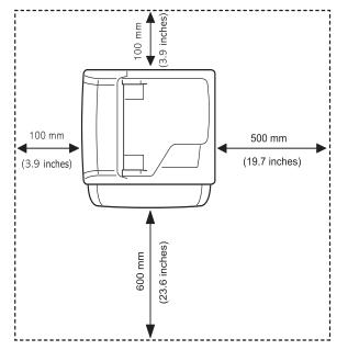
A horizontal plane must be within 5 mm (0.02 inches) both from front to rear and from right to left.
